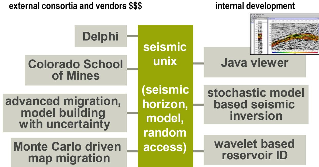
Figure 1. Structure of software. Backplane of seismic unix with a common Java based viewer. Vendors and consortia can add modules. Internal developed propriety or openSource modules can easily be added.
