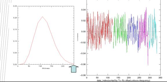
Inversion gives thickness pdf with mean 110m, and 250m above upper 5% quantile.
